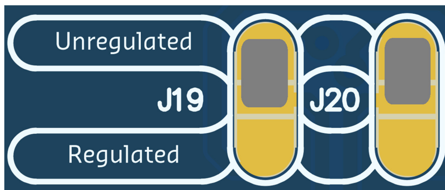
Figure 5. Solder jumpers are located on the bottom side. Grey rectangles indicate default configuration.
